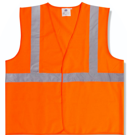
#V220 orange & #V221 yellow/lime This Type R, Class 2, safety vest is constructed of polyester solid fabric and features two-inch reflective tape hook & loop closure
